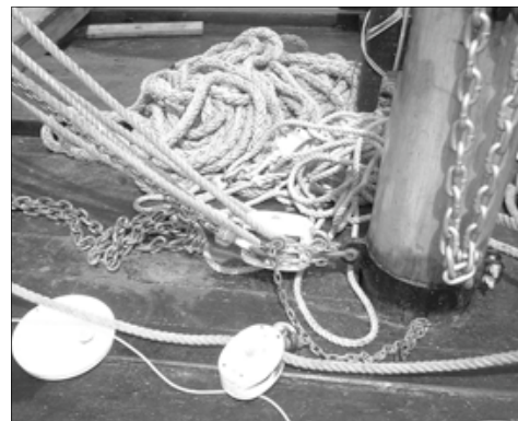
The Adams ’ stump mast was tapered to measure 14” at the base and 12” at the top.
