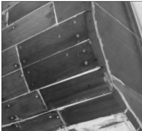
Mahogany planks of varying lengths will replace the rotted sideboards on the Gone with the Wind . Part of the transom, or stern, was full of rotted oak.
