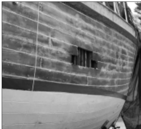
Mahogany planks of varying lengths will replace the rotted sideboards on the Gone with the Wind . Part of the transom, or stern, was full of rotted oak.
